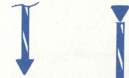
ARROWS SHOW CURRENT FLOW FROM POWER TO GROUND
