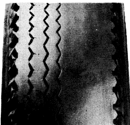
INCORRECT TOE-IN OR EXTREME CAMBER
