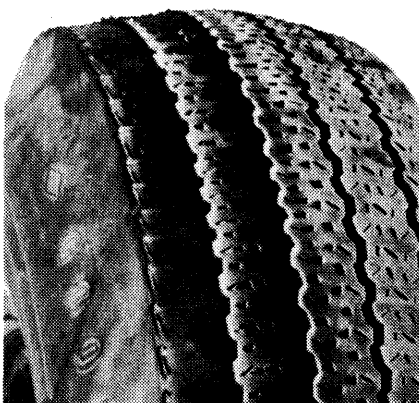
FEATHERING DUE TO MISALIGNMENT OR SEVERE CORNERING
