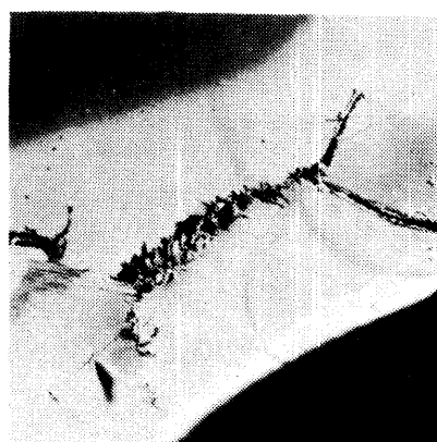
DOUBLEBRUISE—SHARP OBJECT AND RESULTING FATIGUE F1467-D
