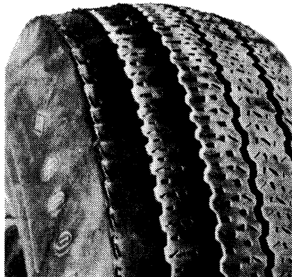
FEATHERING DUE TO MISALIGNMENT OR SEVERE CORNERING
