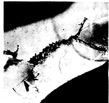
DOUBLEBRUISE—SHARP OBJECT AND RESULTING FATIGUE
