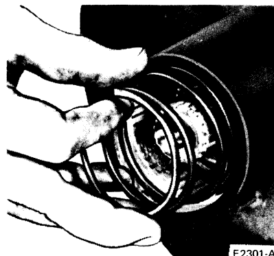
FIG. 9 Coil Spring Installation
