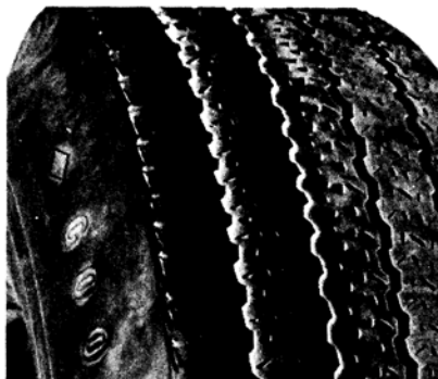
FEATHERING DUE TO MISALIGNMENT OR SEVERE CORNERING
