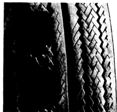
CUPPING—UNDERINFLATION AND/OR MECHANICAL IRREGULARITIES
