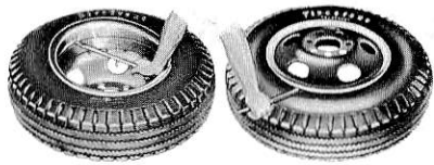
FIG. 3 Removing Ring and Removing Tire—Two-Piece Rim
