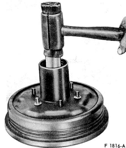
FIG. 26 Inner Bearing Cone and Grease Seal Removal
