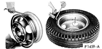
FIG. 2 Removing Ring and Loosening Tire Bead—Two-Piece Rim
