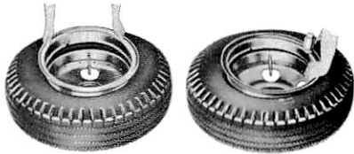
FIG. 4 Positioning and Starting Ring—Two-Piece Rim
