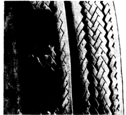
CUPPING—UNDERINFLATION AND/OR MECHANICAL IRREGULARITIES
