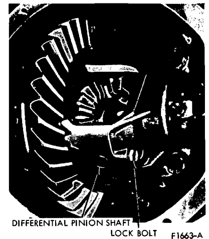
FIG. 5 Differential Pinion Shaft and Lock Bolt
