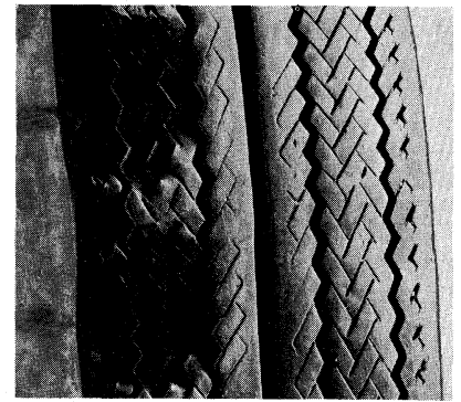
CUPPING—UNDERINFLATION AND/OR MECHANICAL IRREGULARITIES
