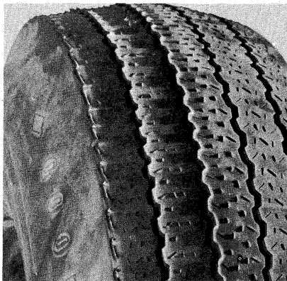
FEATHERING DUE TO MISALIGNMENT OR SEVERE CORNERING
