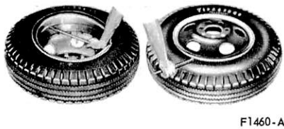
FIG. 4—Removing Ring and Removing Tire—2—Piece Rim
