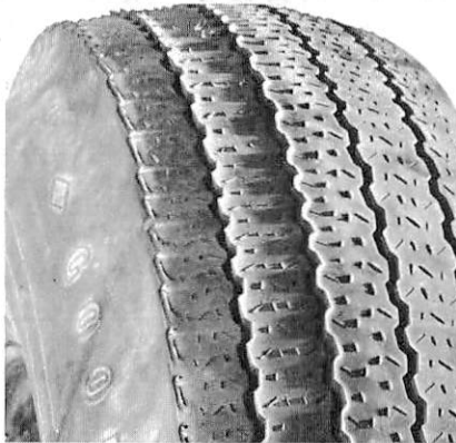
FEATHERING DUE TO MISALIGNMENT OR SEVERE CORNERING
