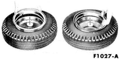
FIG. 5—Positioning and Starting Ring—2—Piece Rim
