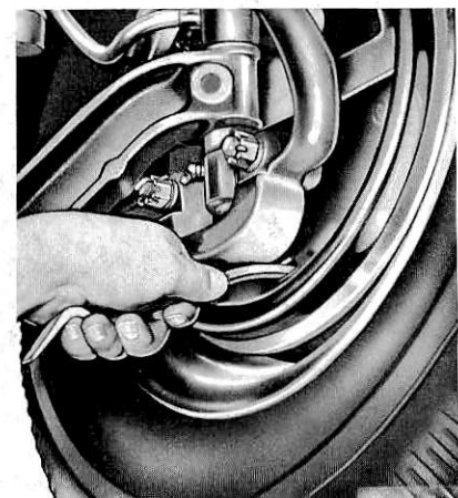
FIG. 11—Single Anchor Brake Shoe Adjustment
