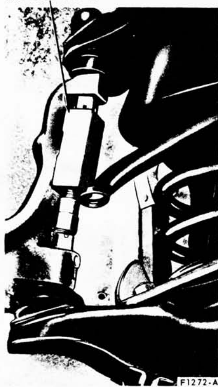
FIG. 3—Disconnecting the Ball Joints—Typical
