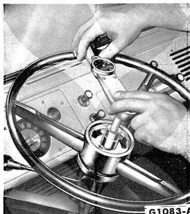
FIG. 3—Checking Steering Gear Preload
