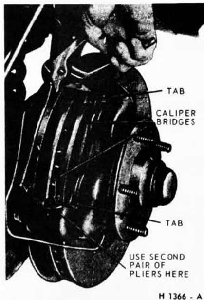
FIG. 7—Removing Disc Brake Shoe and Lining Assembly
