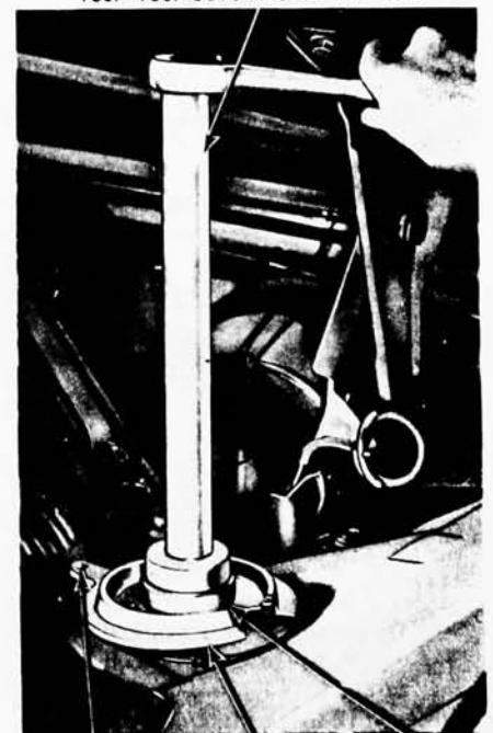
FIG. 6 – Compressing or Releasing Spring—Upper View
