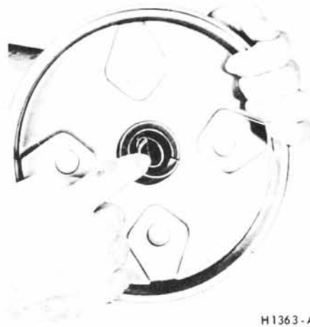
FIG. 22—Removing or Installing Rear Seal to End Plate
