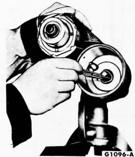
FIG. 30—Removing Piston O-Ring
