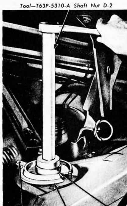
FIG. 6—Compressing or Releasing Spring—Upper View
