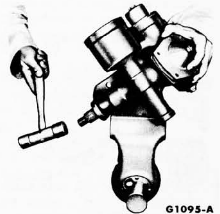
FIG. 29—Removing Sector Shaft
