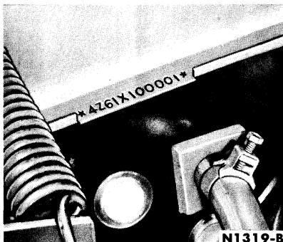
FIG. 2—Ford Vehicle Identification Number Location
