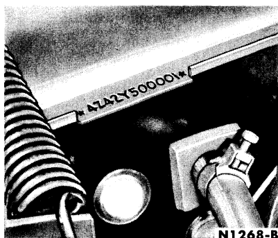
FIG. 4—Mercury Vehicle Identification Number Location
