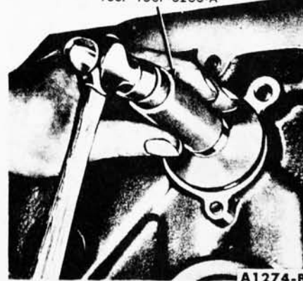
FIG. 91—Camshaft Rear Bearing Bore Plug Installation
