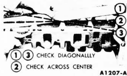
FIG. 37—Cylinder Head Flatness
