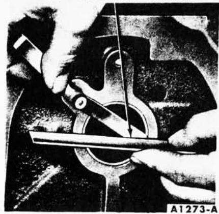
FIG. 90—Camshaft Front Bearing Measurement
