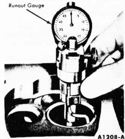
FIG. 38—Valve Seat Runout
