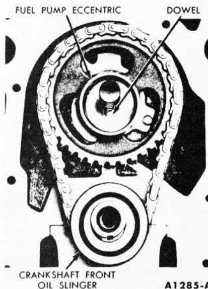
FIG. 58—Fuel Pump Eccentric and Front Oil Slinger Installed
