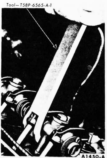
FIG. 50—Bleeding Down Hydraulic Valve Lifter
