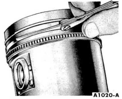
FIG. 22—Piston Ring Side Clearance
