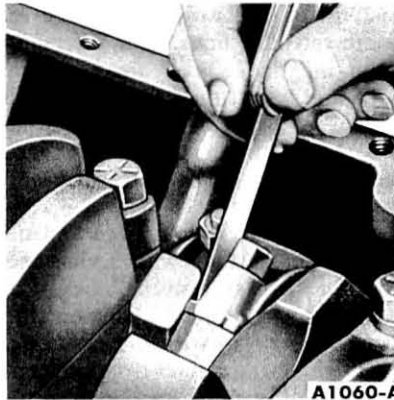
FIG. 33—Checking Side Clearance
