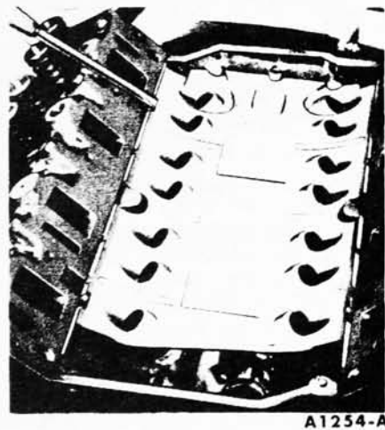
FIG. 16—Baffle Plate Removal
