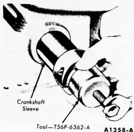
FIG. 20—Crankshaft Sleeve Removal
