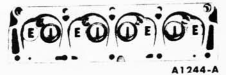
FIG. 6—Valve Port Arrangement
