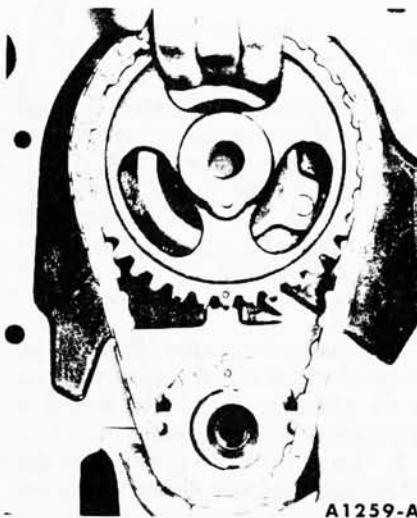
FIG. 21—Timing Chain Removal or Installation
