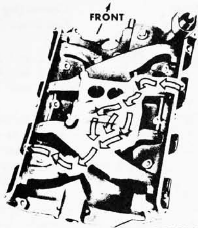
FIG. 3—Intake Manifold Exhaust Gas Passages
