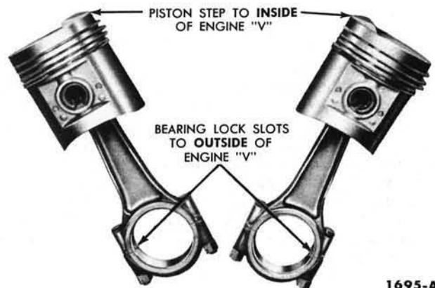
FIG. 46—Connecting Rod and Piston Assembly
