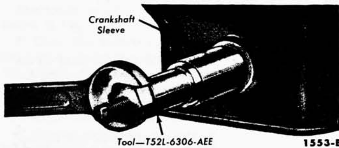
FIG. 48—Crankshaft Sleeve Installation
