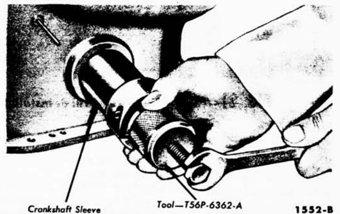
FIG. 20—Crankshaft Sleeve Removal
