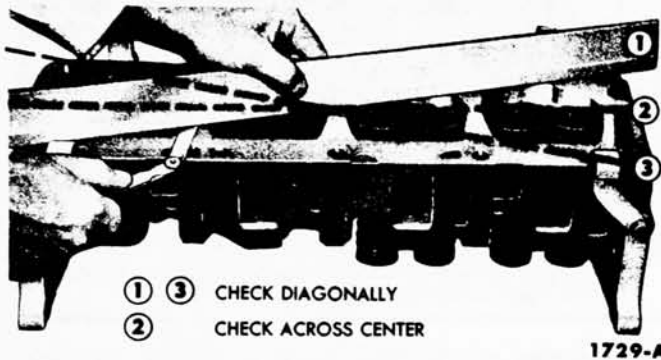
FIG. 5—Cylinder Head Flatness—Typical
