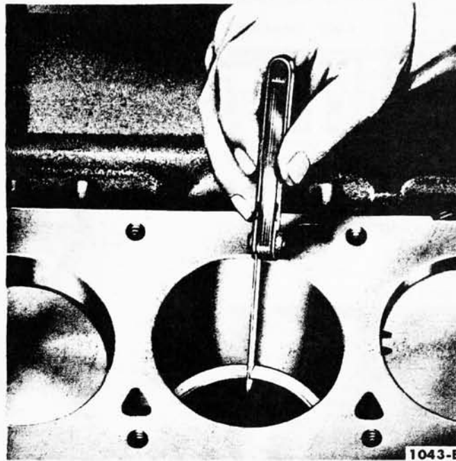
FIG. 20—Piston Ring Gap—Typical
