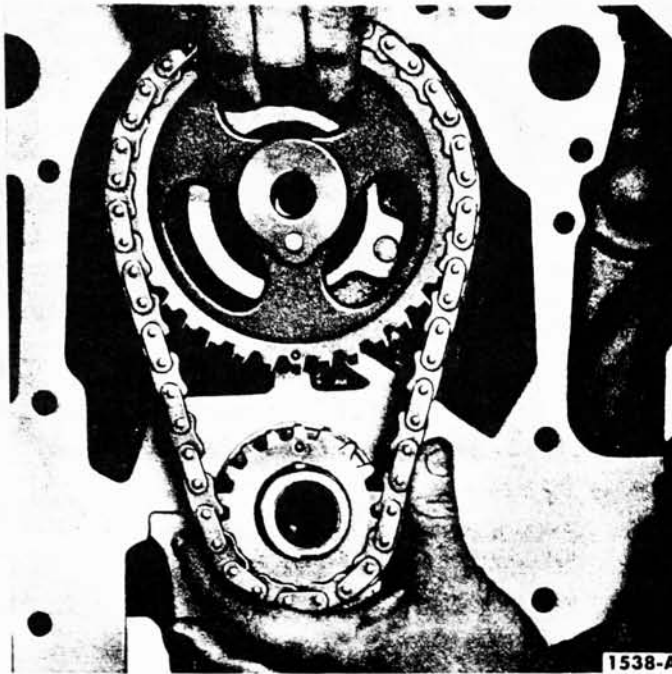
FIG. 21—Timing Chain Removal or Installation
