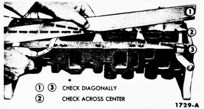
FIG. 62—Cylinder Head Flatness
