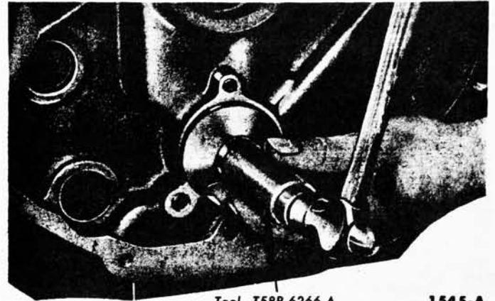
FIG. 27—Camshaft Rear Bearing Bore Plug Installation
