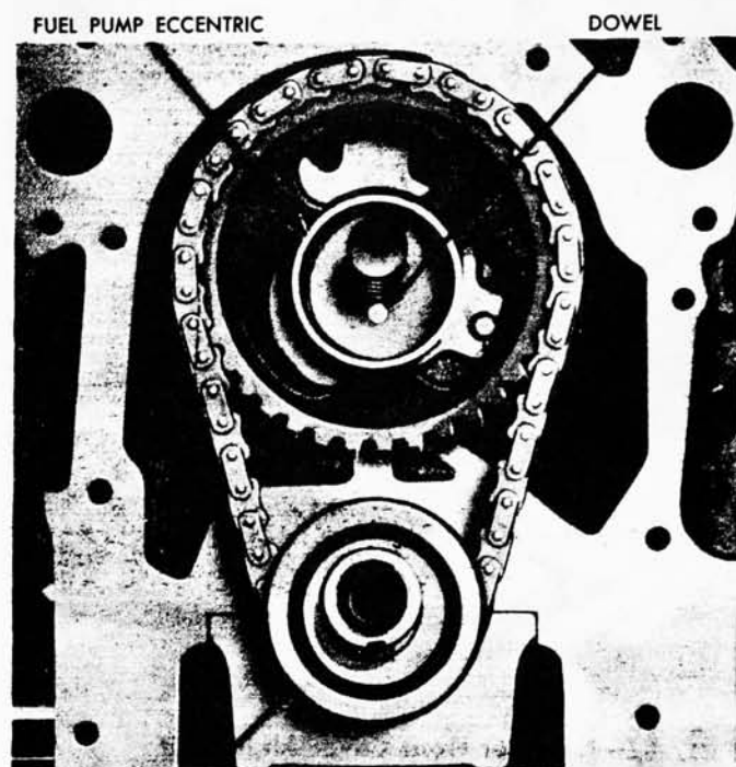
FIG. 40—Fuel Pump Eccentric and Front Oil Slinger Installed
