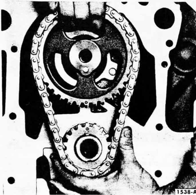
FIG. 24—Timing Chain and Sprockets Removal or Installation
