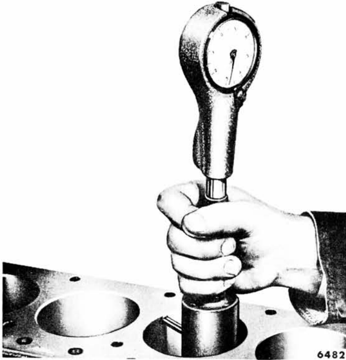
Fig. 35—Cylinder Bore Measurement—Typical
