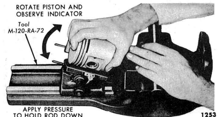
Fig. 57—Check Connecting Rod Alignment
