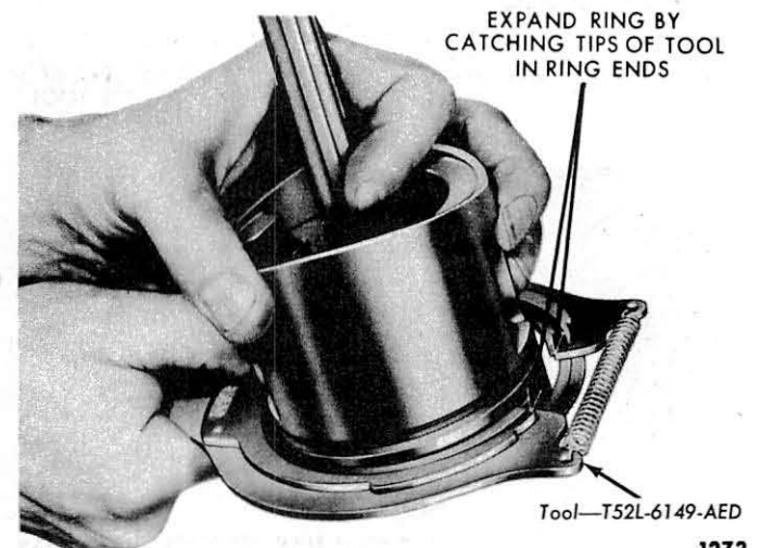
Fig. 53—Removing Rings
