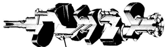
SLUDGE TRAPS (DRILLED IN EACH JOURNAL—INDIVIDUAL OIL PASSAGES FROM SLUDGE TRAP TO EACH ROD BEARING—PRESSED-IN HOLLOW PLUGS SEAL OPENINGS.)
