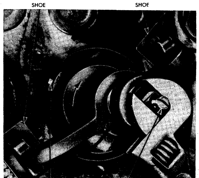
SHOE SHOE CUTTER BLADE PILOT ADJUSTING SCREW 1153 Fig. 64—Removing Cylinder Ridge
