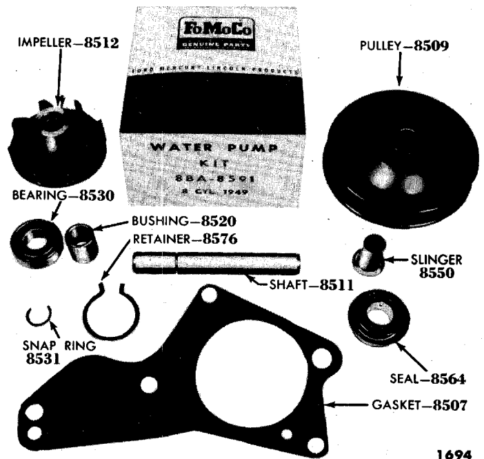
Fig. 68—Early 1949 8-Cylinder Water Pump Repair Kit
